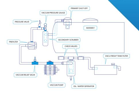
**Application:** Filter odors that are exhausted from the vacuum pump on sewage pump trucks during operation.
